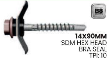
TO STEEL PURLINS UP TO 4.5MM THICK
