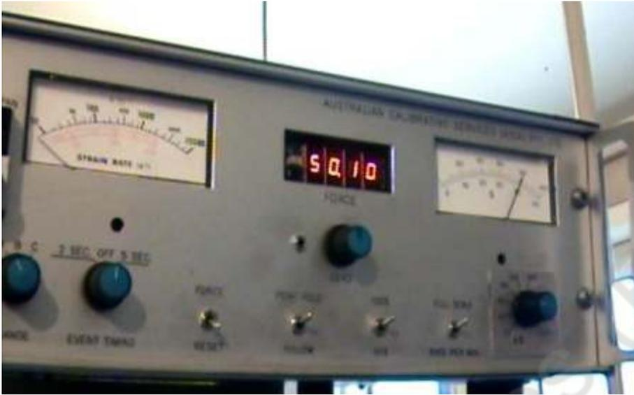
Testing of the SE015HP anchor to 50.1kN.
