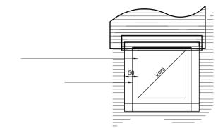
Vent seal against flashing
