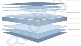
Finish Coat (Finish Coat + Primer = nominal 25 $\mu$ m) {Refer Notes 4 & 5} Universal Corrosion Inhibitive Primer
