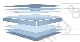
Finish Coat (Finish Coat + Primer = nominal 25μm) {Refer Notes 1, 4 & 5} Universal Corrosion Inhibitive Primer
