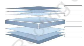
Finish Coat (Finish Coat + Primer = nominal 25µm) {Refer Notes 4 & 5} Universal Corrosion Inhibitive Primer Conversion Coating
