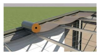
1. Lay Kingspan AIR-CELL perpendicular to purlins ensuring a 50 mm overlap into the gutter.
