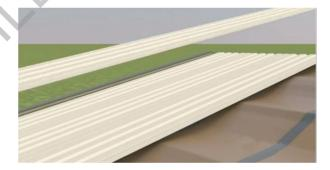
5. Fix roof sheeting by screwing through **Kingspan AIR-CELL** to the purlin.
