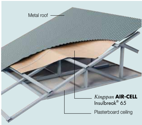
Figure 1 Kingspan AIR-CELL Insulbreak® 65 in a metal roof with a flat ceiling
