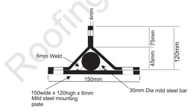
The SE105HP-2PBP bracing plate can be used on both timber and steel structures
