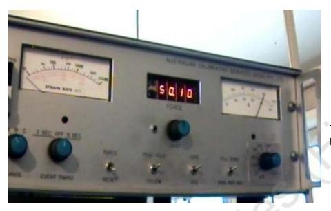
Testing of the SE015HP anchor to 50.1kN.
