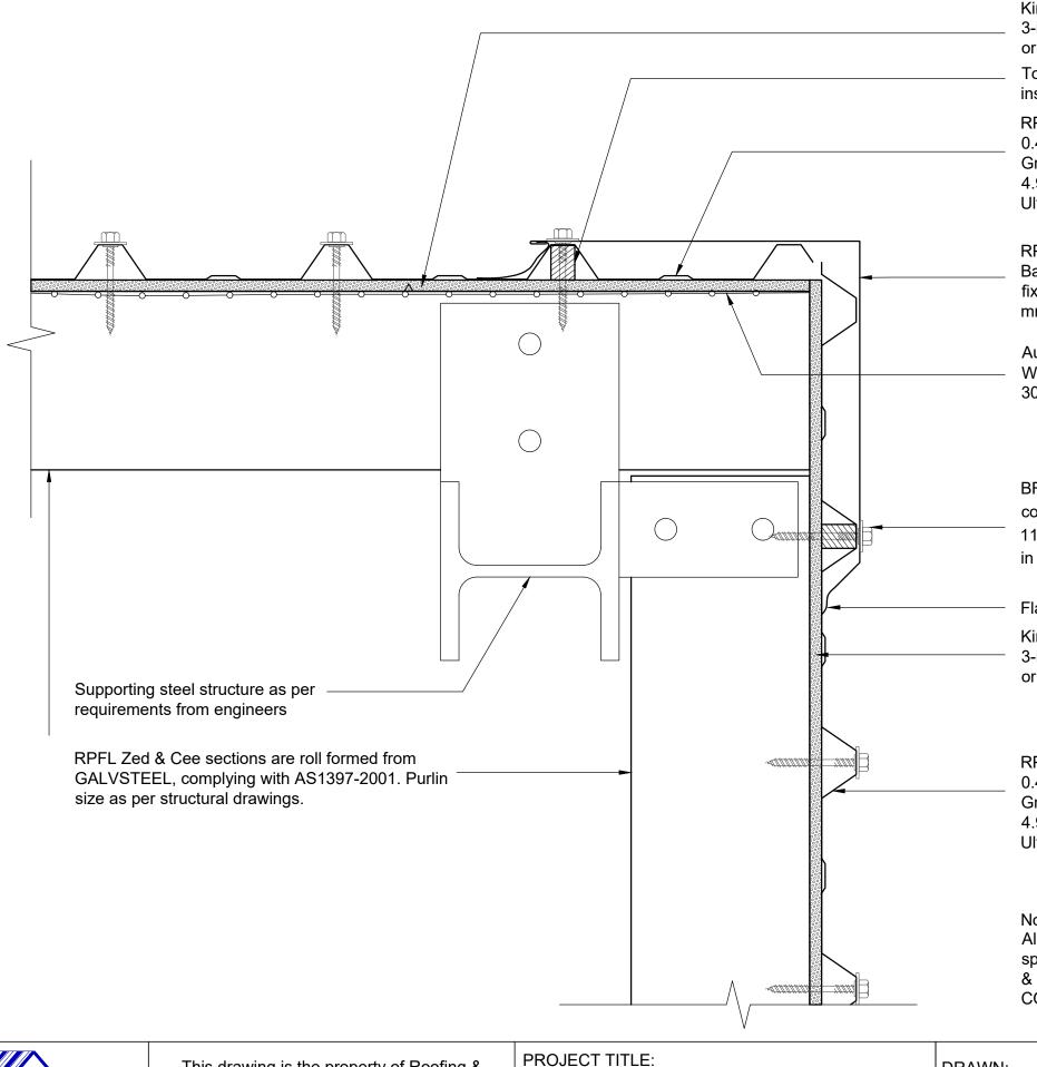
Kingspan AIR-CELL INSULINER Self-Supported 3-in-1 Insulation Vapour Barrier and Radiant Barrier or 430 WF Med. duty sisalation
