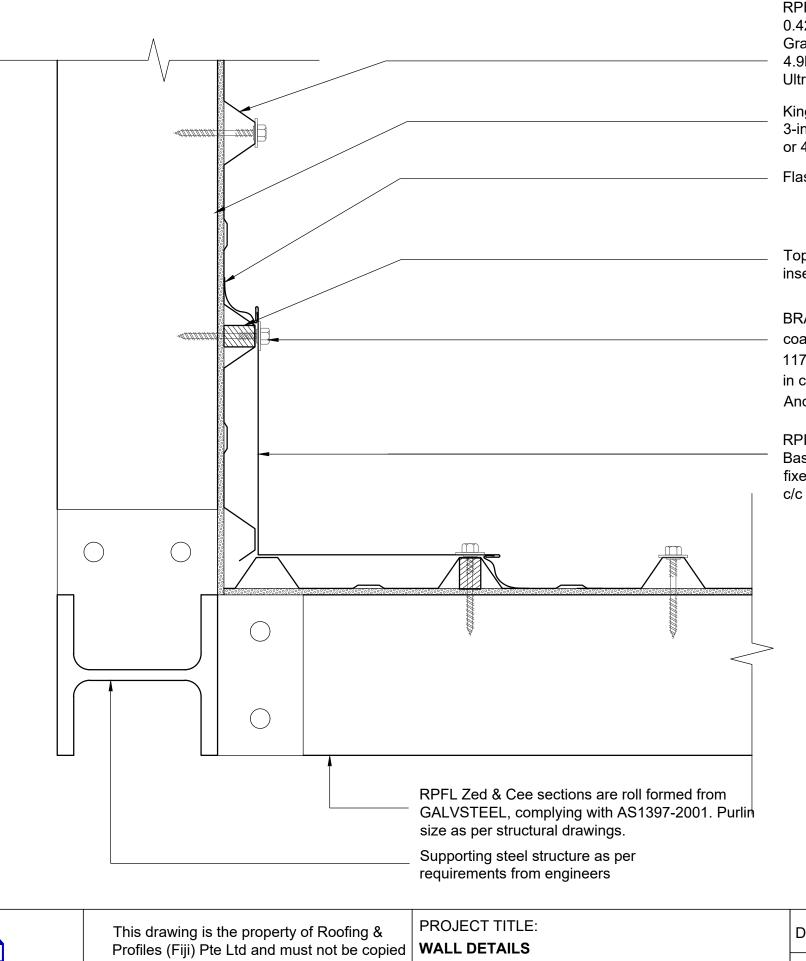
RPFL SuperDek® Colorbond® XRW/Ultra 0.42BMT/0.48BMT wall cladding. Base Materials: Steel Grade G550. BMT 0.42.Mass 4.3kg/m2 or 0.48BMT 4.9kg/m2. AZ 150 coating for XRW & AZ 200 coating for Ultra. Profiles tested for Cyclonic Conditions.
