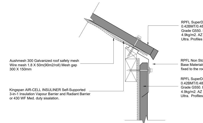
RPFL SuperDek® Colorbond® XRW/Ultra 0.42BMT/0.48BMT Roof cladding. Base Materials: Steel Grade G550. BMT 0.42.Mass 4.3kg/m2 or 0.48BMT 4.9kg/m2. AZ 150 coating for XRW & AZ 200 coating for Ultra. Profiles tested for Cyclonic Conditions.
