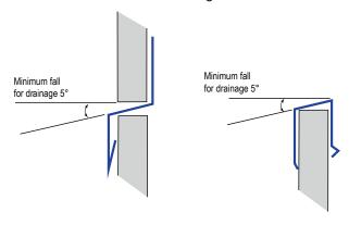
ed using self drilling screws or rivets. Fixing as close as possible Flashing is fix
