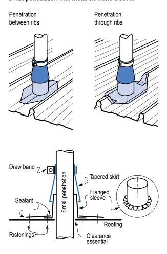
Figure 3.13.2 Small penetration with sleeve. (Dektite®sleeve illustrated).
