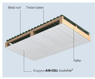
Figure 1 Kingspan **AIR-CELL** Insulwhite<sup>®</sup> in a pitched metal roof retrofit installation (attic conversion)
