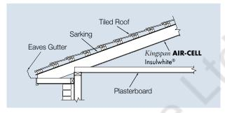
Figure 4 Side elevation of *Kingspan* **AIR-CELL** Insulwhite<sup>®</sup> in a pitched tiled roof retrofit (attic conversion)
