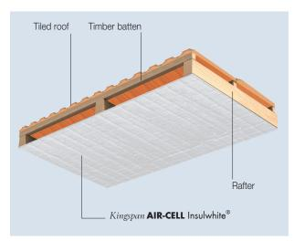
Figure 3 Kingspan **AIR-CELL** Insulwhite<sup>®</sup> in a pitched tiled roof retrofit installation (attic conversion)
